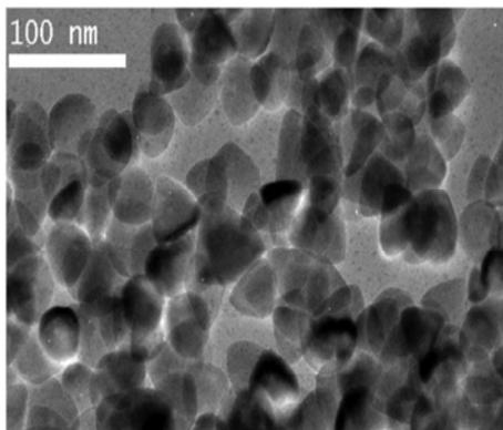
Fig. 3: TEM picture of vanadium-doped zinc oxide nanopowder.
