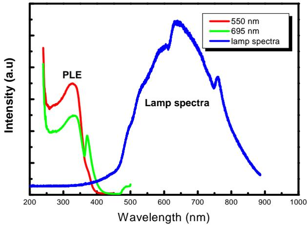
Fig. 5: Intersection between lamp spectra and PLE spectra.
