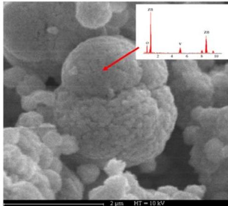
Fig. 2: SEM image of vanadium-doped zinc oxide powder and EDX analysis
