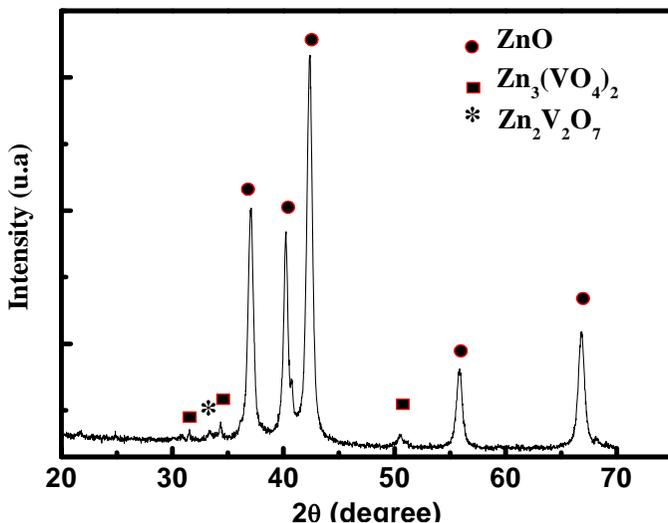
Fig.1: X-ray diffraction of nanoparticles powder of ZnO:V.
